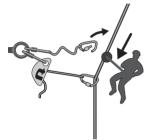
With rescue loads in descent, this can be physically difficult. Prepare in advance by fitting two deviations in parallel, one slightly shorter than the other and with the shorter link releaseable (e.g. using a descender or slip knot to lock it off).
