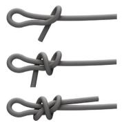
Tied identically to one half of a double fisherman's bend, but starting with a bight of rope.
