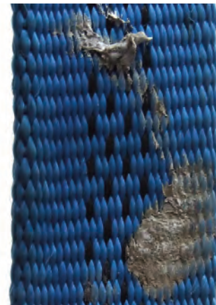
Silicone rubber sealant marks on a webbing sling - harmless.
